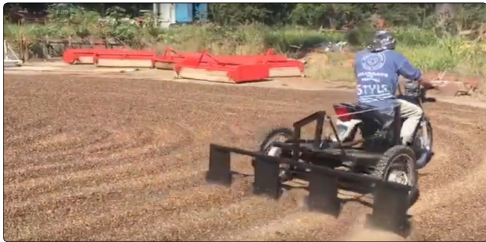
Figure 2. Motorcycle adapted for drying coffee in the patio.
