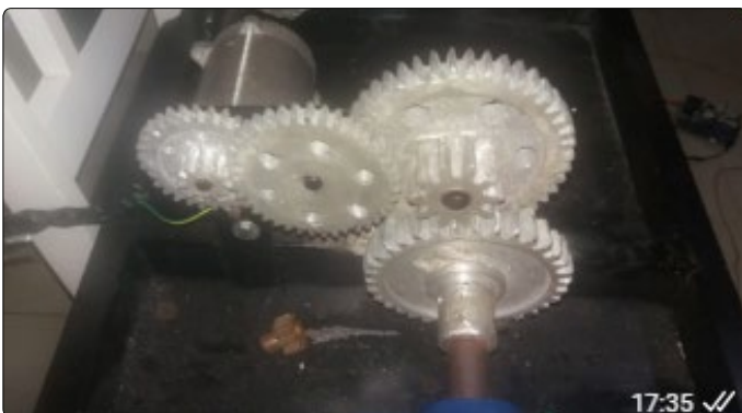
Figure 7. Gearbox coupled to the motor.
