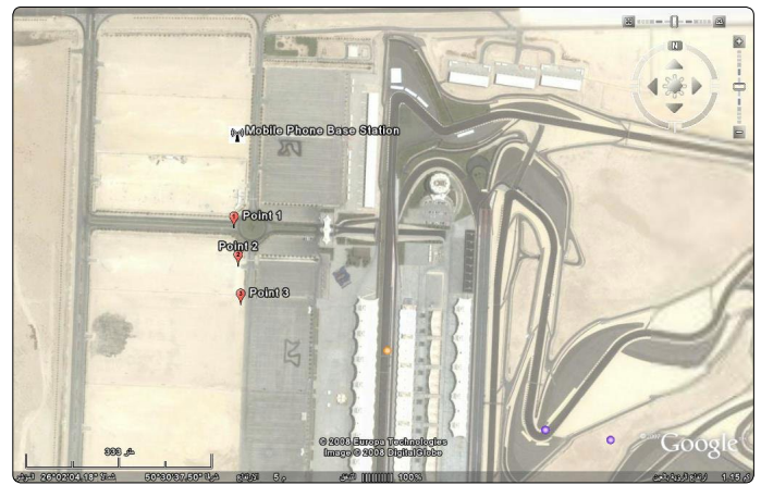
Figure 2. An aerial photo showing the locations of the points of measurement (160 m, 230 m and 300 m) of the level of EMR from the mobile base station at BIC, Kingdom of Bahrain.
