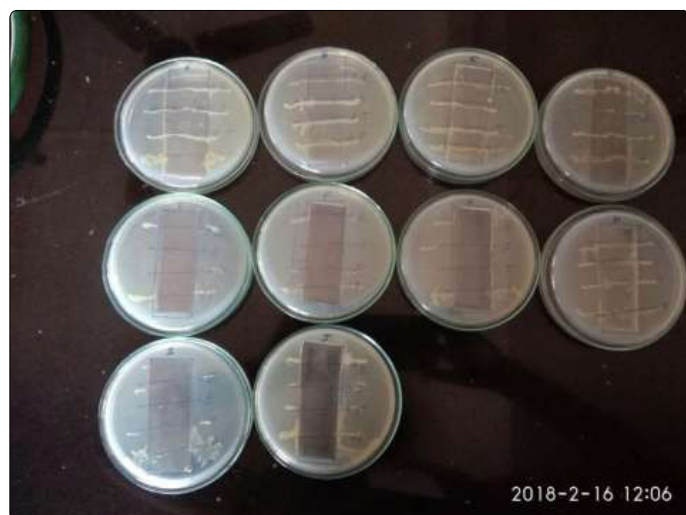
Figure 7. Images of antimicrobial Inhibition for A-( \text{Sn}_{0.02}, \text{Sr}_{0.08} : CdS), B-( \text{Sn}_{0.04}, \text{Sr}_{0.06} : CdS), C-( \text{Sn}_{0.06}, \text{Sr}_{0.04} : CdS), D-( \text{Sn}_{0.08}, \text{Sr}_{0.02} :CdS), E-Pure CdS, F-( \text{Sn}_{0.02}, \text{Sr}_{0.08} : ZnS), G-( \text{Sn}_{0.04}, \text{Sr}_{0.06} : ZnS), H-( \text{Sn}_{0.06}, \text{Sr}_{0.04} : ZnS), I-( \text{Sn}_{0.08}, \text{Sr}_{0.08} ZnS) and J- pure ZnS respectively.
