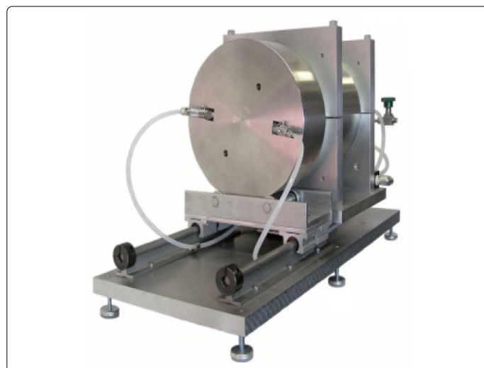
Figure 2. Custom built high pressure high temperature oven used for the pyrolysis of SiCN.
