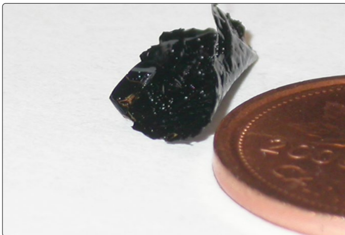
Figure 11. Curling of thin film SiCN. Thin films of SiCN may curl after cooling as thermal stress is expected to be encountered. Any variation in structure yields to non-homogeneity throughout the thickness of the structure. When the temperature drops, the differential shrinkage rate yields curling of thin (5 \mu\text{m} thick) SiCN
