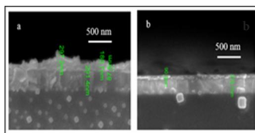
Fig 2. SEM cross-sectional images of (a) Ru(II)-MEPE thin film (b) pretreated Ru(II)-MEPE thin film.
