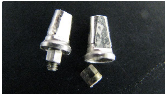
Figure 6. An abutment fractured under overload and/or excessive tightening with its intact original.
