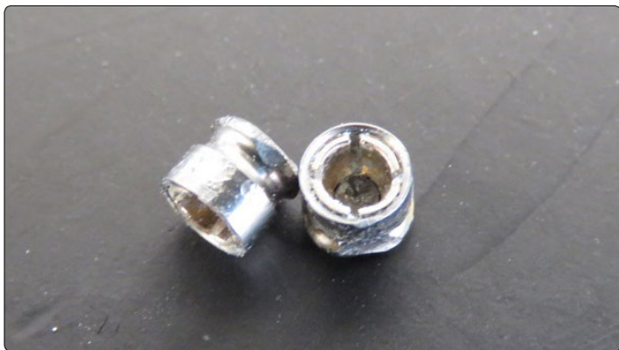
Figure 4. Precision attachment females an implant-retaining overdenture failed due to the harmful effects of non-parallel path of insertion.
