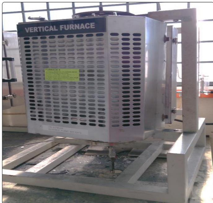
Figure 1. Stainless steel vertical tubular furnace
